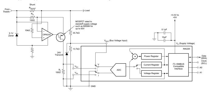
Figure 32. 48-V Telecom Current/Voltage/Power Sense
