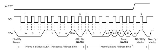
NOTE (1): The value of the Slave Address Byte is determined by the settings of the A0 and A1 pins. Refer to Table 1.
