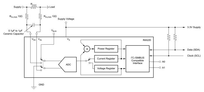
Figure 14. INA220 With Input Filtering
