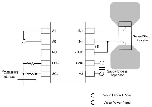
(1) Connect the VBUS pin to the power supply rail
