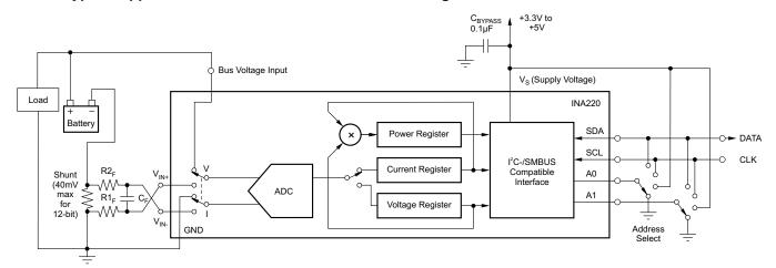
Figure 33. General Source Low-Side Sensing
