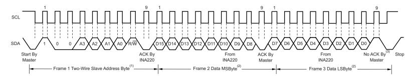
NOTES: (1) The value of the Slave Address Byte is determined by the settings of the A0 and A1 pins. Refer to Table 1.
