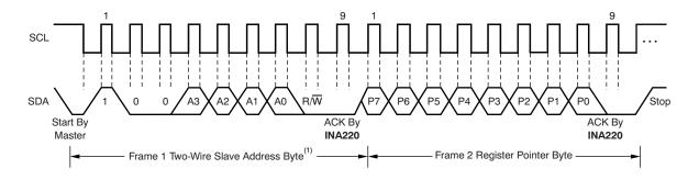
NOTE (1): The value of the Slave Address Byte is determined by the settings of the A0 and A1 pins. Refer to Table 1.
