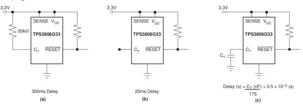
Figure 8-2. Configuration Used to Set the RESET Delay Time
