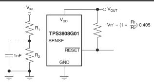
Figure 8-1. Using the TPS3808G01 to Monitor a User-Defined Threshold Voltage
