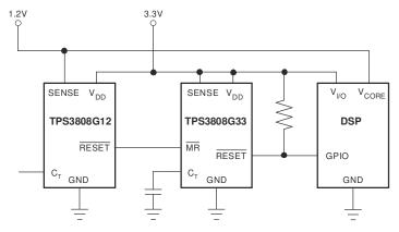
Figure 8-3. Using MR to Monitor Multiple System Voltages
