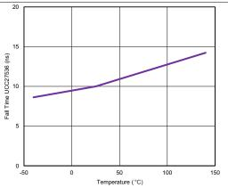
$C_{LOAD} = 1.8 \text{ nF}$   $V_{DD} = 18 \text{ V}$
