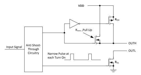
Figure 39. UCC27531 Gate Driver Output Stage
