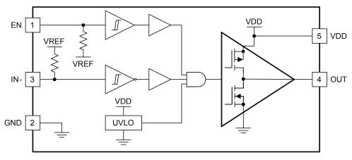
EN Pull-Up Resistance to VREF = 500 k $\Omega$ , VREF = 5.8 V, IN- Pull-Up Resistance to VREF = 500 k $\Omega$
