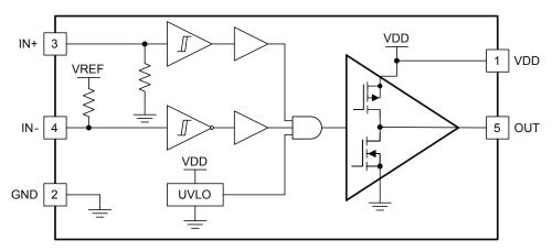
IN– Pull-Up Resistance to VREF = 500 k $\Omega$ , VREF = 5.8 V, IN+ Pull-Down Resistance to GND = 230 k $\Omega$
