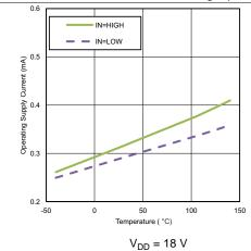
Figure 22. Operating Supply Current vs. Temperature (Output In DC On/Off Condition)
