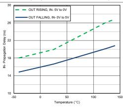
Figure 24. IN- Input-To-Output Propagation Delay vs. Temperature
