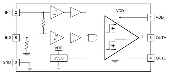
IN1 Pull-Down Resistance to GND = 230 k $\Omega$ , IN2 Pull-Down Resistance to GND = 230 k $\Omega$
