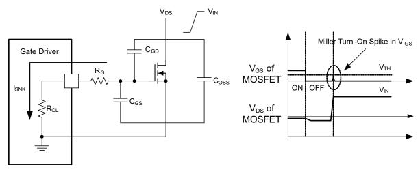
Figure 40. Low Pull-Down Impedance in UCC2753x (Output Stage Mitigates Miller Turn-On Effect)
