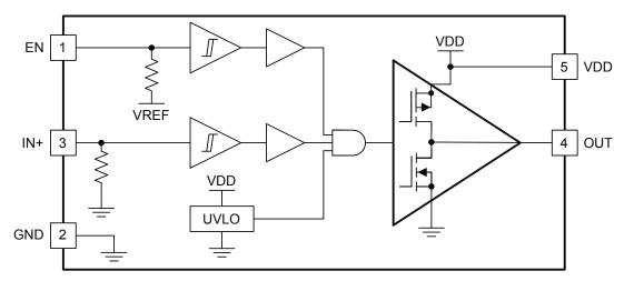
EN Pull-Up Resistance to VREF = 500 k $\Omega$ , VREF = 5.8 V, IN+ Pull-Down Resistance to GND = 230 k $\Omega$
