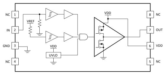
IN Pull-Down Resistance to GND = 230 k $\Omega$ , VREF = 5.8 V, Pull-Up Resistance to VREF = 500 k $\Omega$
