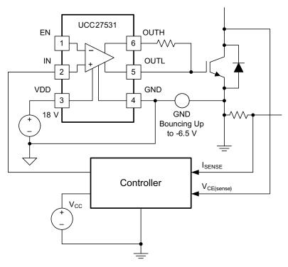
Figure 41. Driving IGBT Without Negative Bias
