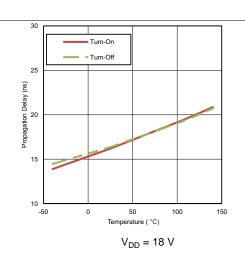
Figure 23. Input-To-Output Propagation Delay vs.
