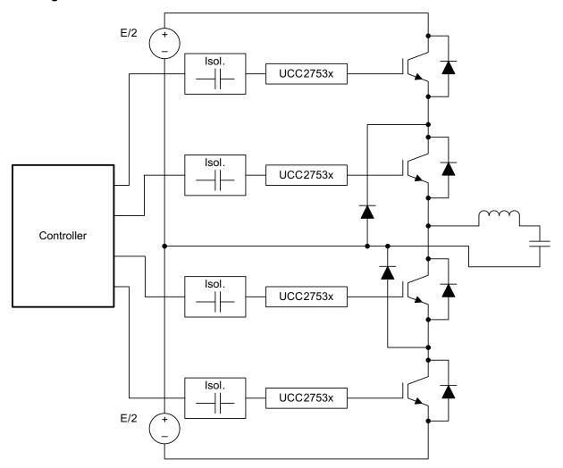
Figure 47. Using UCC2753x Drivers in an Inverter
