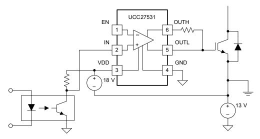
Figure 45. Driving IGBT With 13-V Negative Turn-Off BIAS
