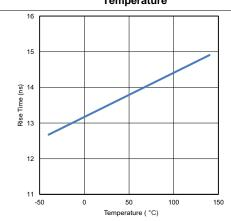
Figure 25. Rise Time vs. Temperature
