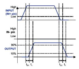
Figure 2. UCC27533: (Output = OUT) Input = IN+ UCC27536: (Output = OUT) Input = EN
