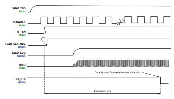
Figure 8-5. Bluetooth-Bluetooth low energy Power-Up Sequence
