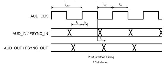
Figure 8-12. Bluetooth Codec-PCM (Audio) Master Timing Diagram
