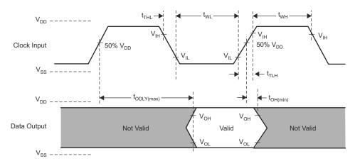
Figure 8-9. SDIO HS Output Timing
