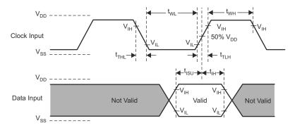
Figure 8-8. SDIO HS Input Timing
