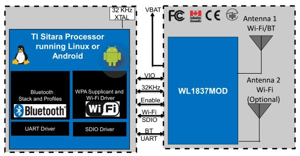
Figure 9-1. WL1837MOD High-Level System Diagram
