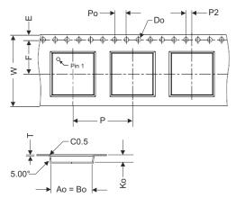
Figure 12-2. Tape Specification
