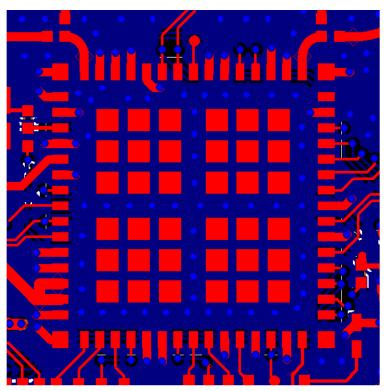
Figure 10-3. TI Module Layout: Layer 1
