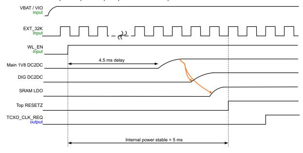
Figure 8-3. Chip Top-Level Power-Up Sequence
