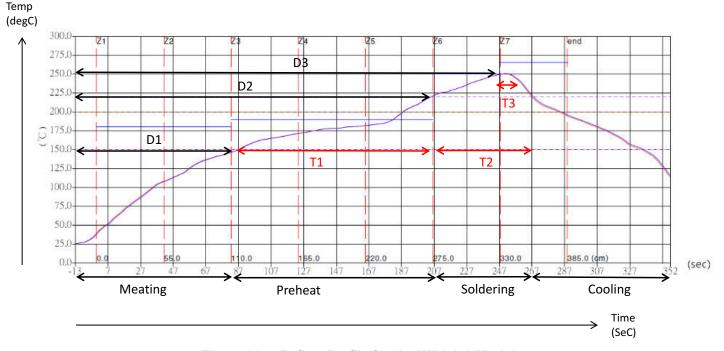
Figure 10-7. Reflow Profile for the WiLink 8 Module
