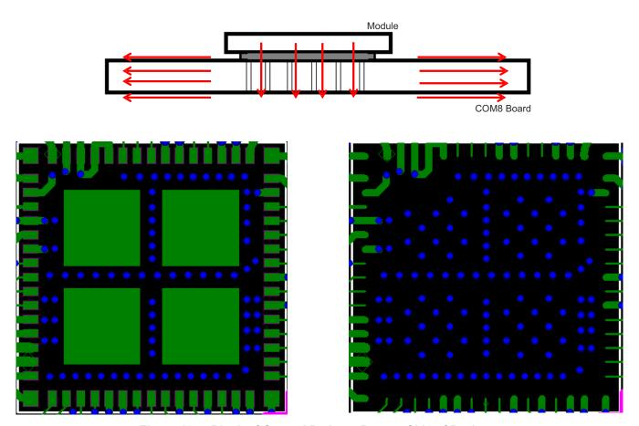
Figure 10-5. Block of Ground Pads on Bottom Side of Package
