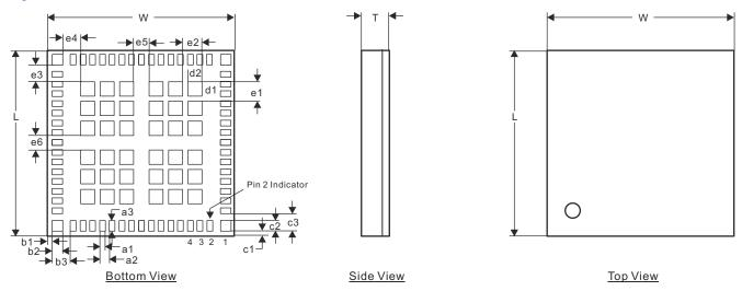
Figure 12-1. TI Module Mechanical Outline
