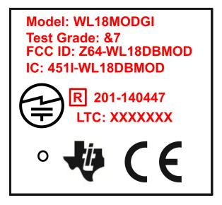
Figure 9-2. WiLink 8 Module Markings
