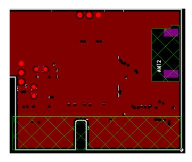
Figure 10-4. TI Module Layout: Layer 2 (Solid GND)
